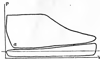
FIG. 204. Art. 463, Prob. 31. — Diagrams from Woolf Engine.
